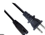
CE033 Power Cord US Type SPT-1,18AWG*2C,OD:2.7*5.4mm 1.5m/1.8m/3m/5m
